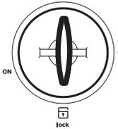
When the key lock switch is in the "OFF" and "LOCK" positions, the compactor will not operate. Remove the key to keep children from operating the unit or to prevent anyone from tampering with it.
