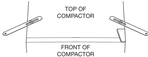
Two under-counter mounting straps are provided. Use these straps to secure the compactor to the underside of a countertop. Fasten the slotted end of the straps to the compactor using the holes in the top of the compactor cabinet as shown.
