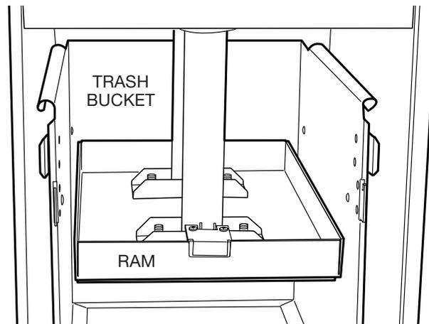
1. Make sure the trash bucket is empty and pushed into the cabinet.
