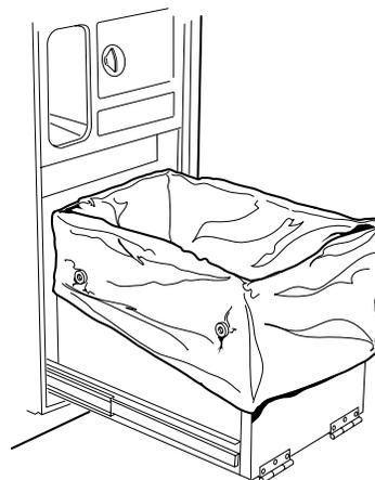
Smooth and shape the bag carefully - this will prevent the bag from being torn by the ram during compaction.
