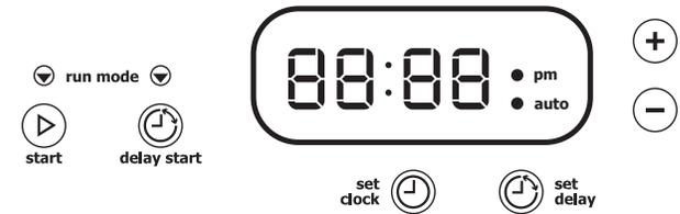
The compactor is equipped with a delay start /clock feature that allows you to compact your trash at a time of your choice (such as every evening).
