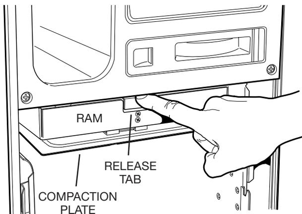
1. The ram is equipped with a compaction plate that can be removed for easy cleaning.
