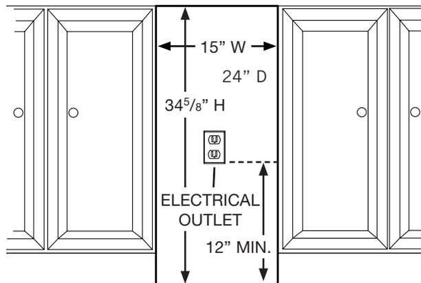
The compactor requires an under-counter opening 15-in. wide, 34<sup>5</sup>/<sub>8</sub>-in. high, and 24-in. deep.
