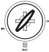
When the key lock switch is in the "ON" position, the compactor is ready for operation. The key cannot be removed when in the "ON" position.
